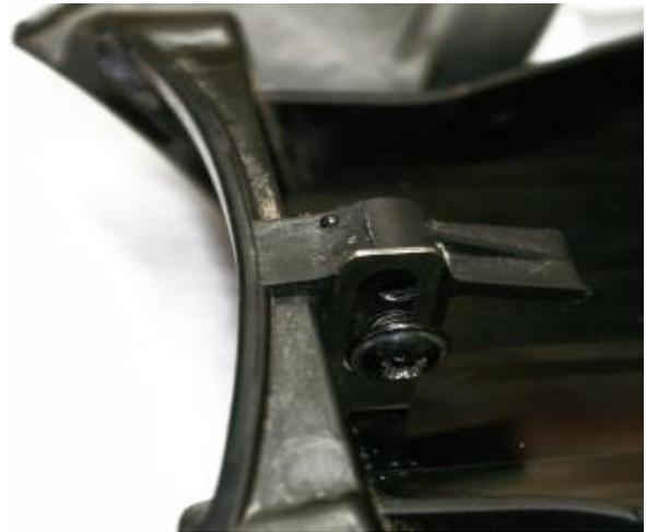
**The photo below represents a proper installation, less your stock rubber straps.**
