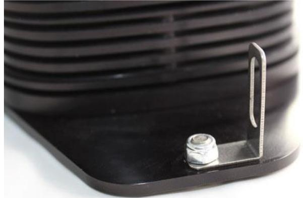
3. Install the top bolt through the strap-extension bracket using the provided M6x18 Button Head Socket Cap bolt. The bracket should be installed on the exterior of the stock plastic tab.
